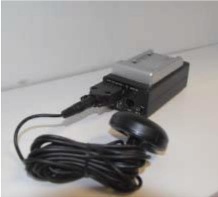
2. Use a male-to-female serial cable to connect the VMS 300 to the COM1 port of the back of your laptop.
